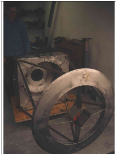
finished optical tube made of stainless steel from welding slightly "dented" before painting
